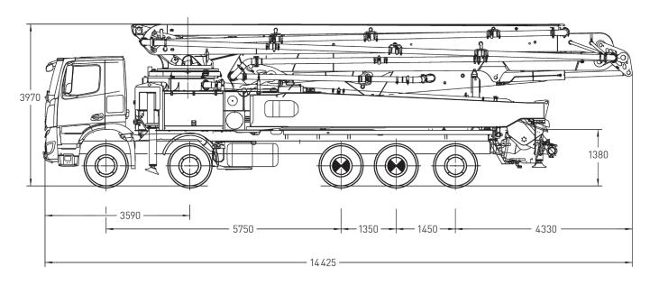
Note: Standard version. Dimensions and weights depend on truck, pump model and equipment. Dimensions in mm, MB-Arocs 4851, Euro 6.
